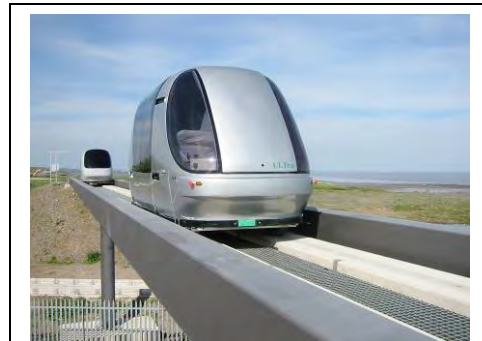
Figure 2. ULTra's elevated open guideway
