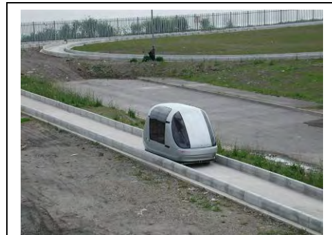
Figure 1. ULTra's at-grade open guideway.
